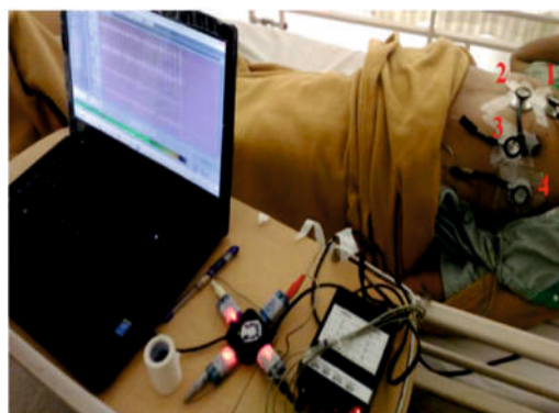
Fig. 7: CAD data acquisition using 4 stethoscopes [11]
